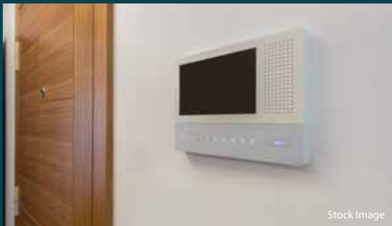
Video Door Phone (VDP) With Intercom Facility From Lobby To Apartment
