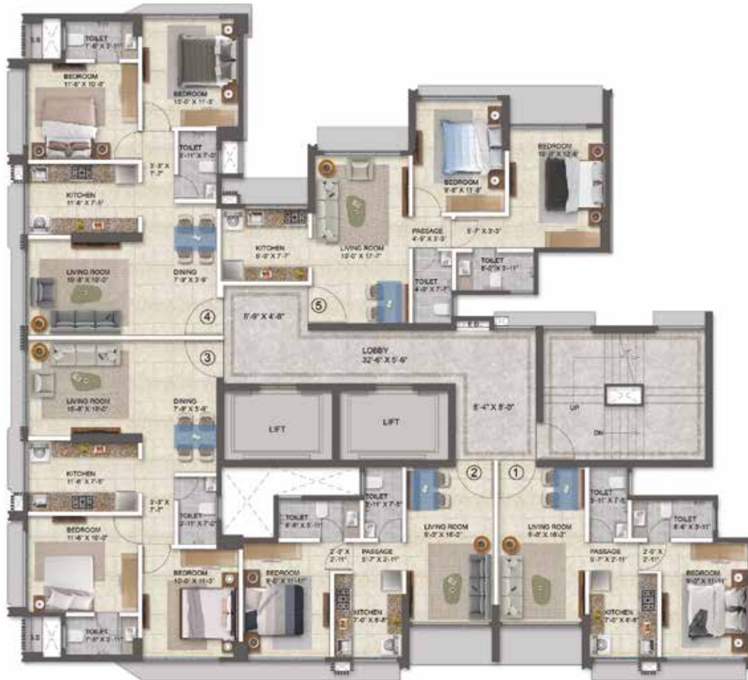
TYPICAL FLOOR PLAN - WING - A 4 TH TO 7 TH , 9 TH TO 13 TH FLOOR
